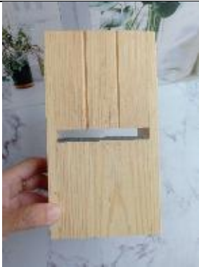
Gambar 7. Soap Beveller/Alat serut sabun
